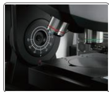
side camera shows the relationship between the lens and the workpiece, reducing the risk of collision
